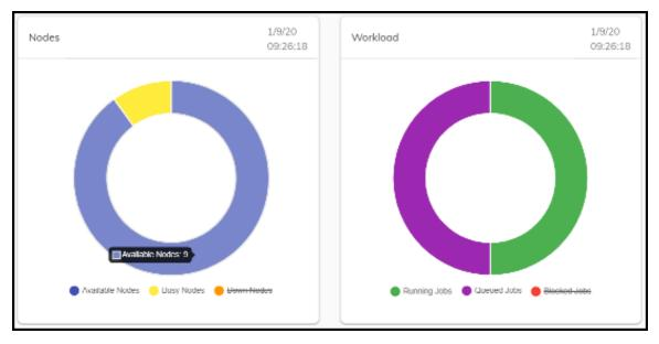
This graph shows the status of Available Nodes, Busy Nodes, & Down Nodes, and the status of the Running Jobs, Queued Jobs, & Blocked Jobs. Click to deselect nodes and jobs to narrow the display results. Hover over the graph to see the number of nodes or jobs.
