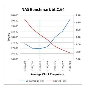
So turning off the node or slowing the clock frequency whenever excess CPU time is available is one sure way to lower energy consumption. Of course, there are power-performance tradeoffs, but certain jobs, such as memory-bound workloads, make this strategy potentially advantageous.
